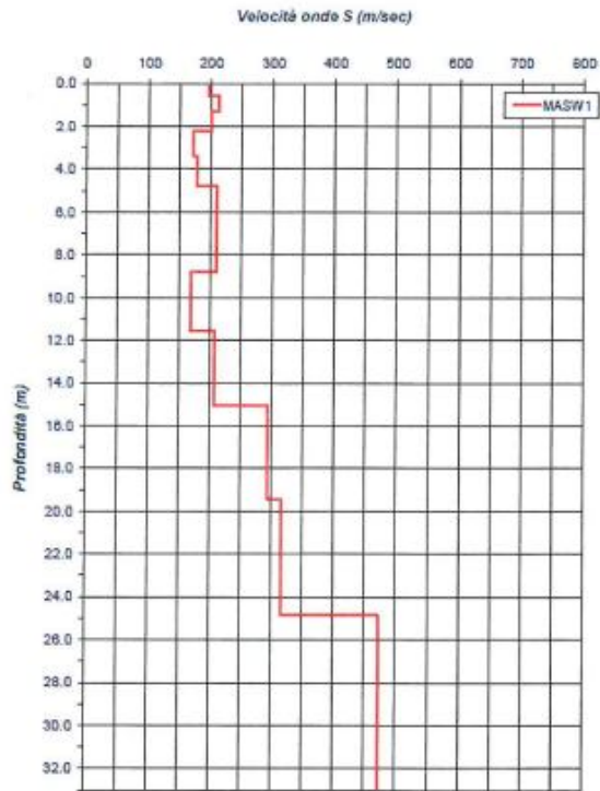
Shear-Wave Velocity Profile from Surface waves inversion
